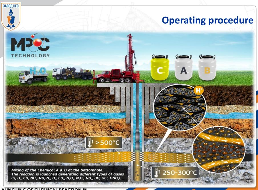
LAUNCHING OF CHEMICAL REACTION IN THE BOTTOM HOLE
